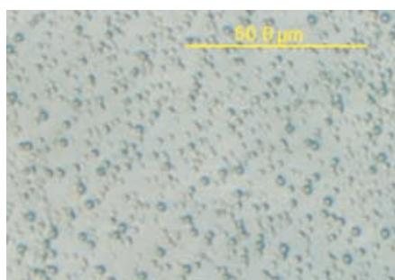
Figure 3. Optical micrograph of a mixture of 1a and 1-phenyl-1-propanol in water at 80°C.
